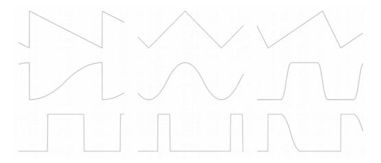
The waveform (WF) fader controls the shape of the transition. It changes from a straight ramp (like in triangle or saw), to a sudden change of value (like in a square), passing through a sinusoid shape.
