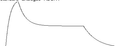
Attack, Decay and Release time, as well as Sustain amplitude can all be adjusted with faders.
