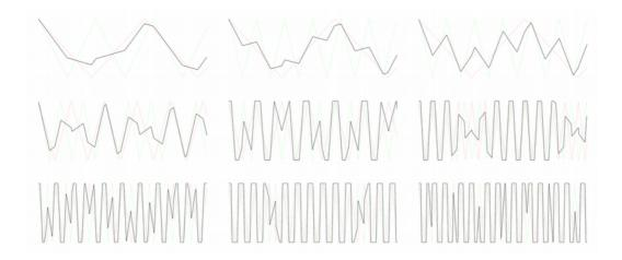
STEP: This LFO generate steps. The FQ fader control the frequency of the steps.
