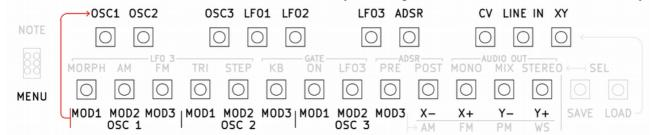
This allow to change the oscillator modulation source, as well as the modulation mixed by the joystick in it's 4 direction (X-, X+, Y-, Y+).
