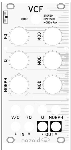
Parametric stereo filter: it can pass from LP to BP and HP in a continuous way
