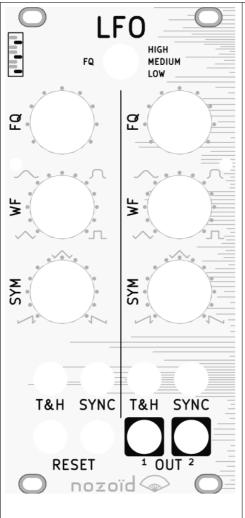
Dual Low Frequency Oscillator, with parametric waveform
