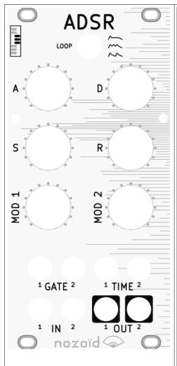
Dual ADSR with modulation speed and integrated VCA
