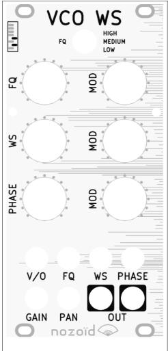
Sinusoidal oscillator with VC waveshaper and VCA and VC Panoramic
