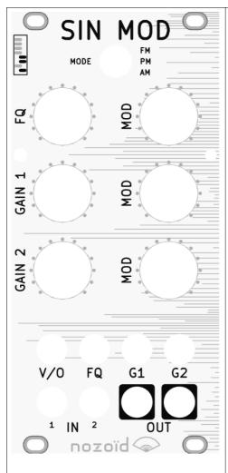
Sinusoidal oscillator with 2 external modulation (PM / FM / AM)
