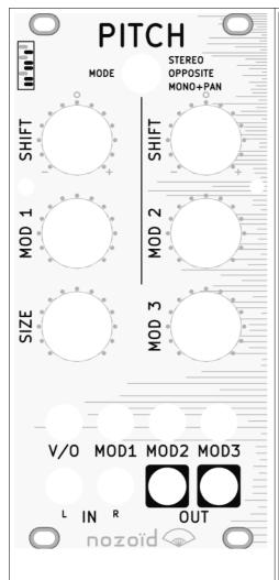
Dual Pitch shifter using tape emulation
