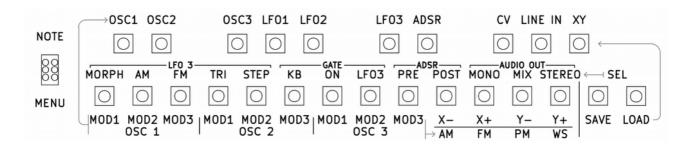
When the toggle is on NOTE, this is a 2 octaves keyboard controlling the frequencies/gate of the VCOs. The portamento filters the frequency change of the keyboard.
