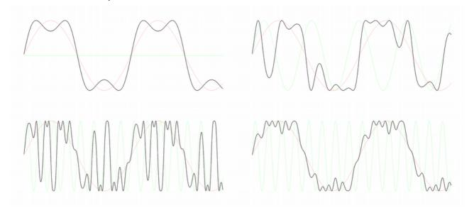
Since an oscillator admit 3 modulation faders, one can use 3 different modulation source with 3 different modulation type, to generate very complex waveform.
