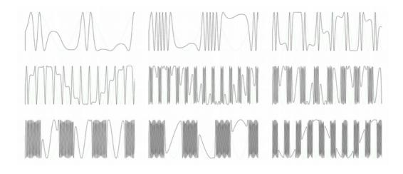
TRI: this LFO mix 2 triangular waveform. The FQ fader control the frequency of the 1<sup>st</sup> triangle waveform. The PARAM 1 fader control the frequency of the 2<sup>nd</sup> triangle waveform. The PARAM 2 fader mix the 2 triangular waveform.
