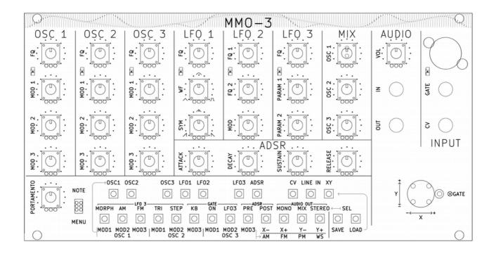
MMO-3 is a digital, semi-modular, monophonic but stereo synthesizer. Built around various types of modulation synthesis, this synthesizer is mostly dedicated to atonal sound generation. From fat drones, glitchy electronic patterns to percussive noise, the MMO-3 offers rich and complex timbre control.
