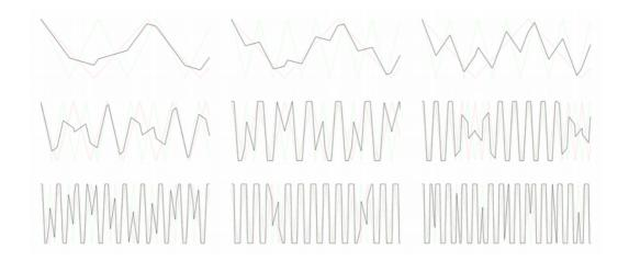
STEP: This LFO generate steps. The FQ fader control the frequency of the steps.
