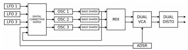
This is the audio path wired inside the synthesizer. Modulation CV are routed to modulation fader in a digital matrix. You will not be short of cable anymore, and you can even save your patch!
